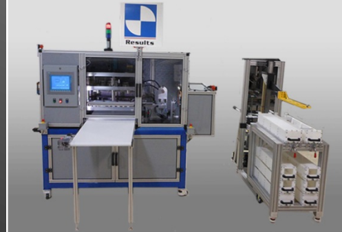
Suture Machine with Custom Hoist
